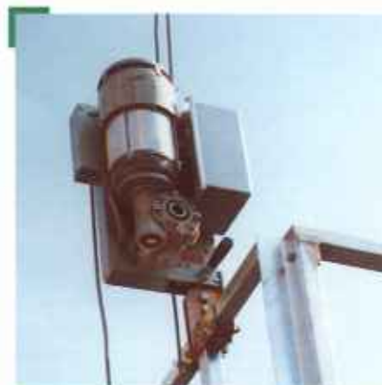
The drive units can also be fixed to the platform ends that are provided with special fixing points. This is a low-cost alternative to C-brackets.
