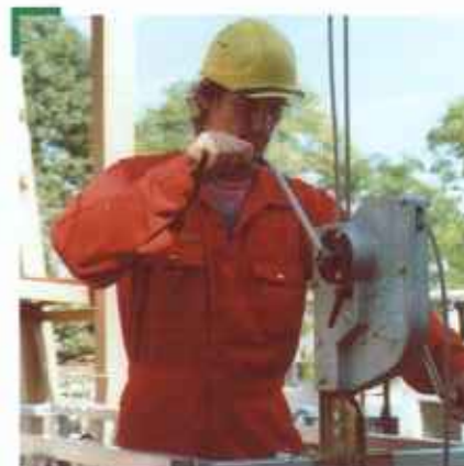
For use in potentially explosive locations a hand drive unit is available as an alternative to the electric version and has proved very effective in these areas.
