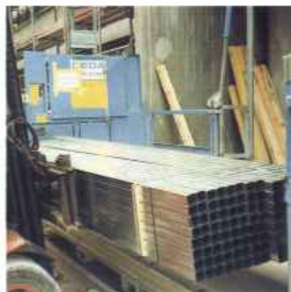
Simple loading of long, bulky material. Load platform variant "I", dimensions 1.65 x 4.35 m.
